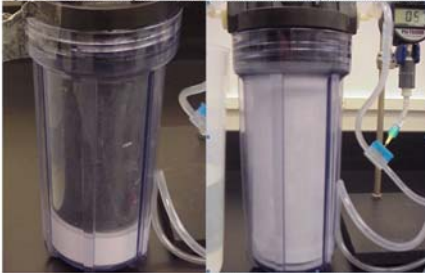
Calcium Phosphate powder dissolves/precipitates to maintain phosphate and calcium levels in dialysate during Whole Body Hyperthermia
